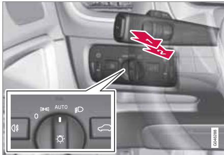
Headlamp control and stalk switch.
