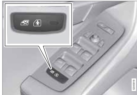
Control panel driver's door.
