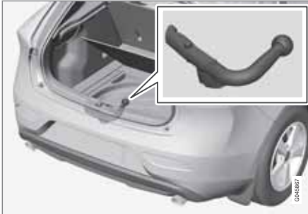
The storage location for the removable towbar.
