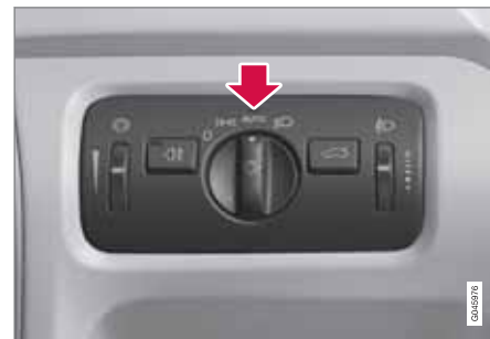
Light switch in position AUTO .
