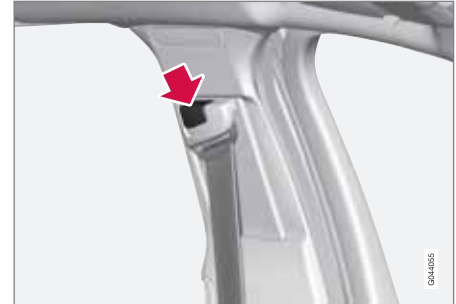
Seatbelt height adjustment. Press the button and move the belt vertically. Position the belt as high as possible without it chafing against your throat.
