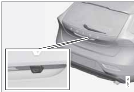
Camera location next to the opening handle.
