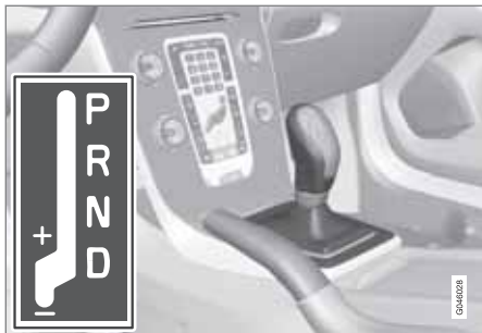
D: Automatic gear positions. +/-: Manual gear positions.
