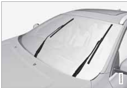
Wiper blades in service position.
