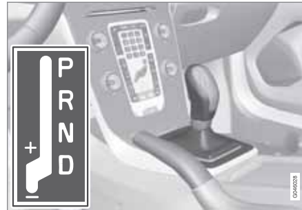
D: Automatic gear positions. +/-: Manual gear positions.
