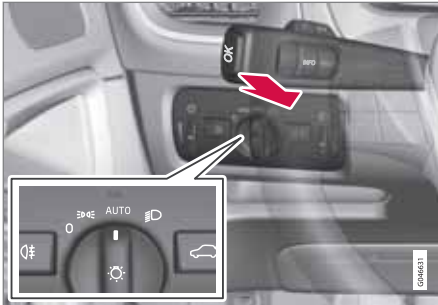
Headlamp control and stalk switch.
