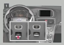
Insert the remote control key in the ignition switch and push in the key to its end position.
