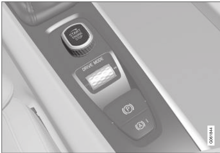
Start knob in the tunnel console.
