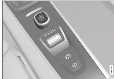
Start knob in the tunnel console.
