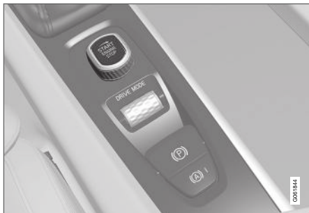
Start knob in the tunnel console.
