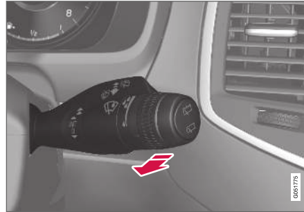
Washing function, right-hand steering wheel lever.
