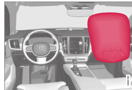
Front passenger airbag in front seat.
