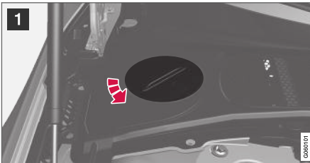
Coolant expansion tank, left-hand drive car.
