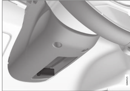
Lever for steering wheel adjustment.
