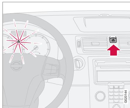
Use the hazard warning flashers (all direction indicators flash) when the car is stopped where it could be a traffic hazard or obstruction. Press the button to activate the function.
