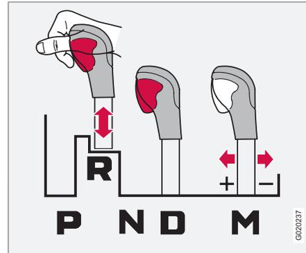
The gear selector can be moved forward and back freely between **N** and **D**. Other positions are locked with a latch that is released with the inhibitor button on the gear selector.
