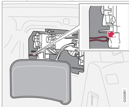
Manual opening of the fuel filler flap is easier when the roof is closed, and is used when it is not possible to open it from the passenger compartment.
