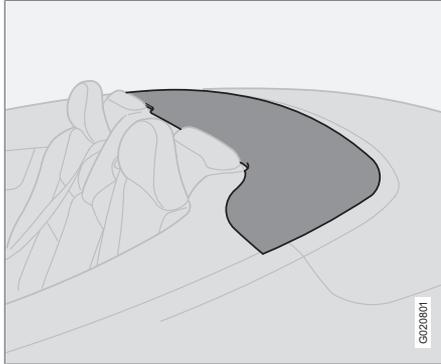
When the roof is open there is a hatch cover between the head restraints in the rear seat and the boot lid, see the preceding illustration.
