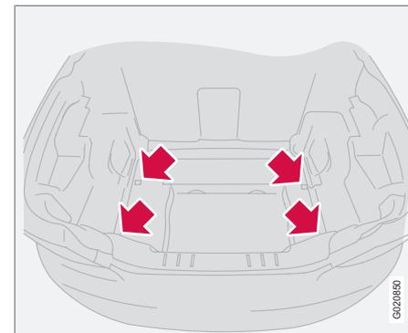
There are four or more eyelets for securing straps or ropes. Straps that are suitable for the eyelets are supplied by Volvo dealers.
