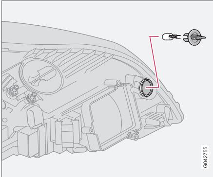
1. Twist the bulb holder anticlockwise and withdraw it. Replace the bulb.
