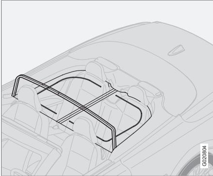
The wind deflector can be used when driving with a lowered roof to reduce the swirling airflow and draughts in the passenger compartment.
