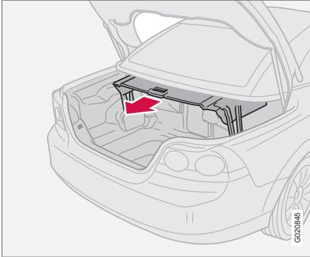
The purpose of the separator is to limit the amount of the load in the cargo area so that the movement of the roof is not disrupted. Be sure to close the cargo separator fully so that it is locked on both the left and right-hand sides.
