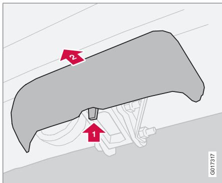
1. Remove the protective cover by first pressing in the catch **1** and then pulling the cover straight back **2**.
