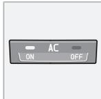
**ON:** The air conditioning is on. It is controlled by the system's AUTO function. This way, incoming air is cooled and dehumidified.
