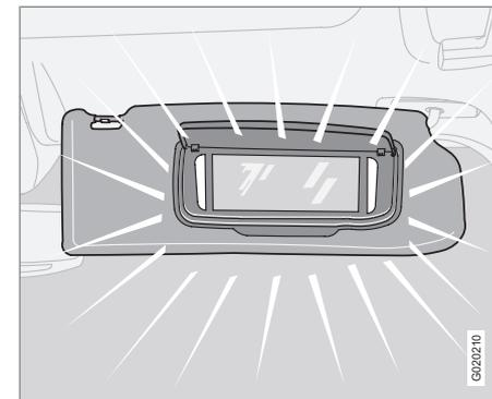
The lamp is automatically switched on and off respectively when the cover is opened or closed.
