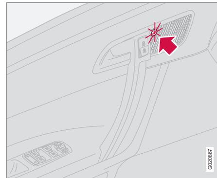
A light on the inside of the door in question illuminates for approx. 5 minutes after the car has been locked with the remote control key's lock button, or with the Keyless drive system when the engine is switched off, see page 126.
