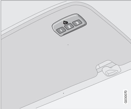
HomeLink®<sup>1</sup> is a programmable remote control which can remotely control up to three different devices (e.g. garage door opener, alarm system, outdoor lighting and indoor lighting etc.) and in doing so replace their remote controls. For more information on HomeLink®, visit: [www.homelink.com](http://www.homelink.com) or ring 00 8000 466 354 65 (or premium rate phone number, +49 6838 907 277).
