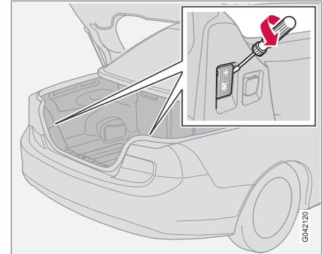
1. Insert a screwdriver and gently turn so that the lamp housing comes loose.
