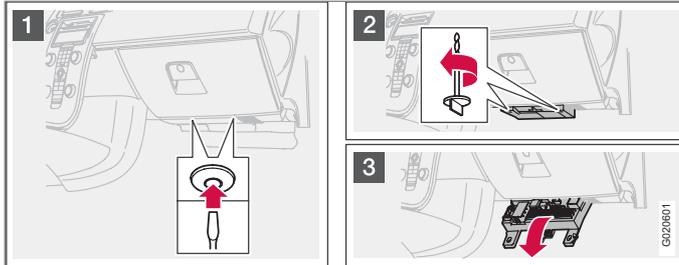
The fuse box has 50 fuse positions. The fuses are located under the glovebox. The box also provides space for several spare fuses. Tools for fuse replacement are located in the relay/fuse box in the engine compartment, see page 228.
