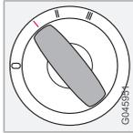
Steering lock deactivated. Certain functions can be used. The engine's electrical system is not activated.
