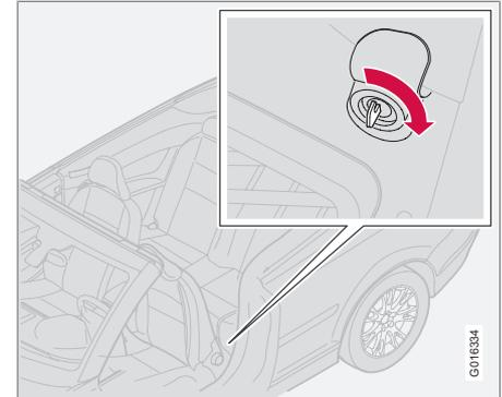
If the car's electrical systems are temporarily out of order then the boot lid can be opened mechanically with the remote control key's detachable key blade. For information on removing the key blade, see page 121.
