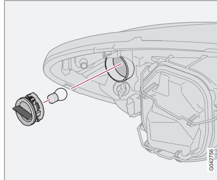
1. Twist the bulb holder anticlockwise and remove it.
