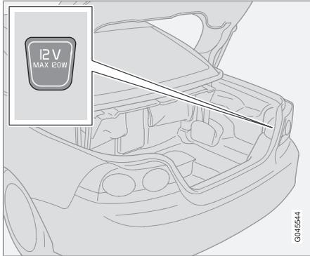
Fold down the cover to access the electrical socket. This socket works regardless of whether or not the ignition is on.
