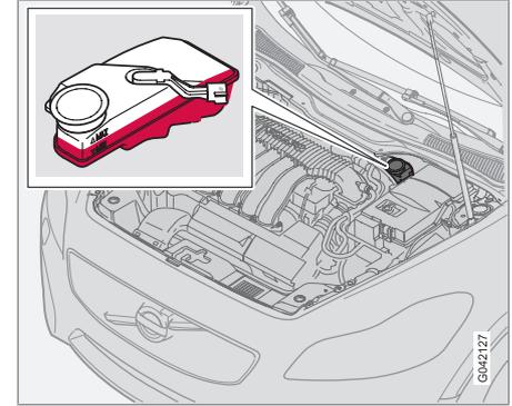
Brake and clutch fluid have a common reservoir<sup>4</sup>. The fluid level must be between the **MIN** and **MAX** marks. Check the level regularly. Change the brake fluid every other year or at every other regular service.
