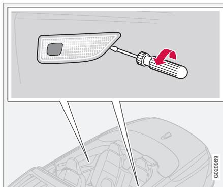
1. Insert a screwdriver and gently turn so that the lamp housing comes loose.
