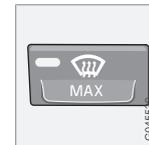
Used to quickly remove misting and ice from the windscreen and side windows. Air flows to the windows at high fan speed. The light in the defroster button illuminates when the function is active.
