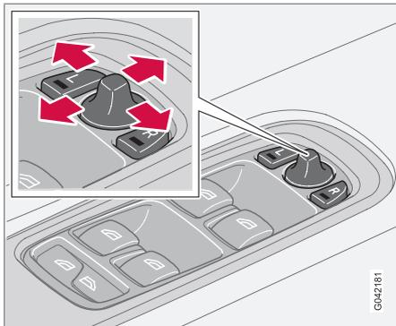
The controls for adjusting the two door mirrors are at the front of the driver's door armrest. The rearview mirrors can be operated in key position I and II.
