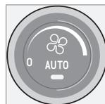
The **AUTO** function automatically regulates climate control and maintains the selected temperature. The AUTO function controls heating, air conditioning, fan speed, recirculation, and air
