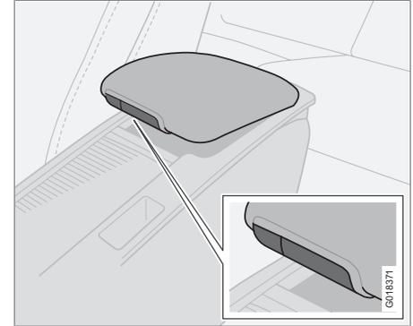
There is a storage space under the armrest. There is also a smaller storage space in the detachable armrest. Press the small button and lift the armrest to open the shallow compartment. Press the large button and lift the armrest to open the deeper compartment.
