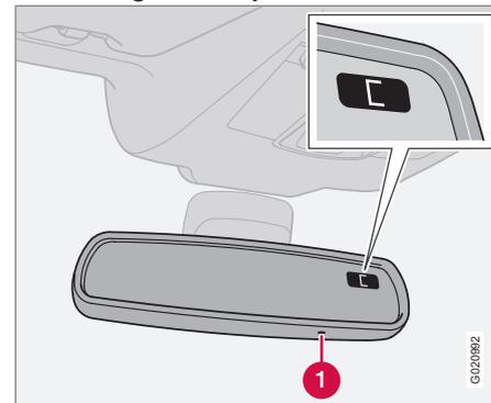
The earth is divided into 15 magnetic zones. The compass is set for the geographical area to which the car was delivered. The compass should be calibrated if the car is moved across several magnetic zones.
