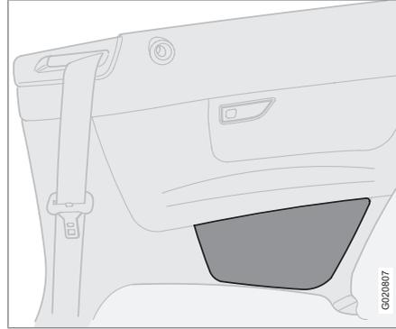
The storage compartment is opened and closed with a touch in the centre of its upper section.
