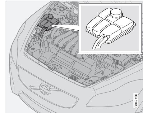
When topping up the coolant, follow the instructions on the packaging. It is important that the mixture of coolant concentrate and water is correct for the prevailing weather conditions. Never top up with water only. The risk of freezing increases with both too little and too much coolant concentrate.
