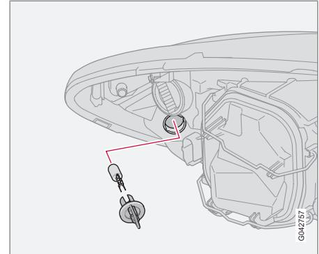
1. Twist the bulb holder anticlockwise and withdraw it. Replace the bulb.
