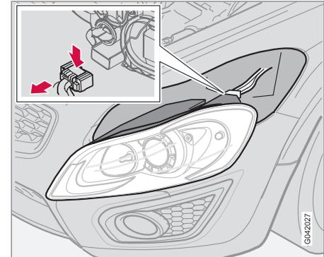
5. Lift out the lamp housing and place it on a soft surface to avoid scratching the lens.
