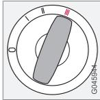
The starter motor is activated. The remote control key is released when the engine has started and then springs back to drive position.
