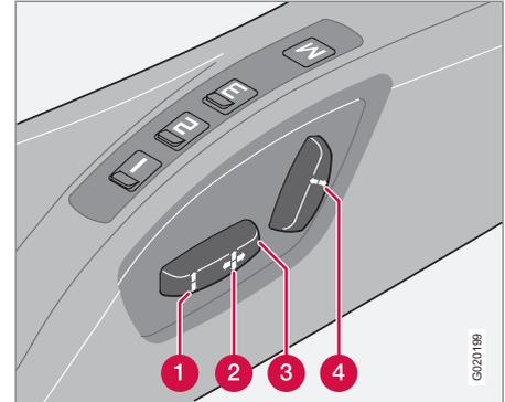
The seats can be adjusted for a certain time after unlocking the door with the remote control key without the key being inserted into the ignition switch. The seat can always be adjusted in key position I or II.
