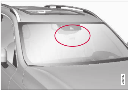
Location of the camera unit.
