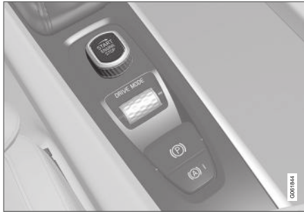
Start knob in the tunnel console.
