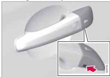
If central locking cannot be activated with the PCC, e.g. if the batteries are discharged, then the driver's door can be opened with the PCC's detachable key blade (see page 49).
