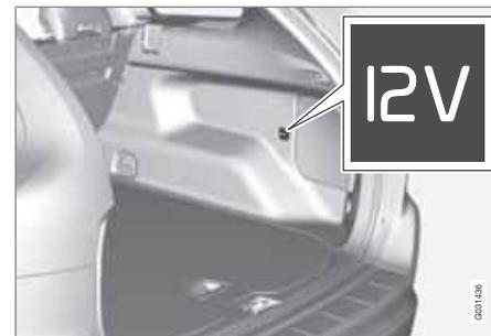
Lower the cover to access the electrical socket. The socket also provides voltage when the remote control key is not in the ignition switch.
