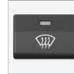
Used to quickly remove misting and ice from the windscreen and side windows. Air flowing to the windows. The light in the defroster button illuminates when the function is active.
