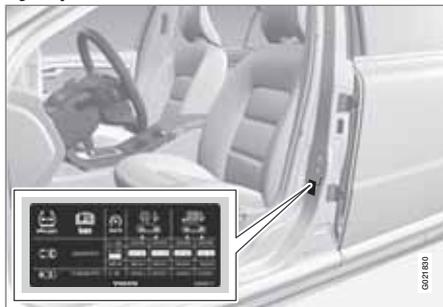
The tyre pressure decal on the driver's side door pillar (between frame and rear door) shows which pressures the tyres should have at different loads and speed conditions. This is also specified in the tyre pressure table, see page 304.
