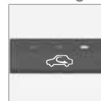
Switch between recirculation On/Off by pressing the button repeatedly. The lamp illuminates when recirculation is engaged.
