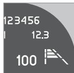
The number of lines for the selected time interval is shown during the setting itself and for several seconds afterwards. Then a smaller scale version of the symbol is shown to the right of the display.
