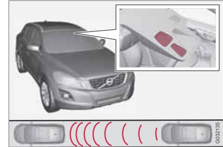
*Laser sensor transmitter and receiver window.*
