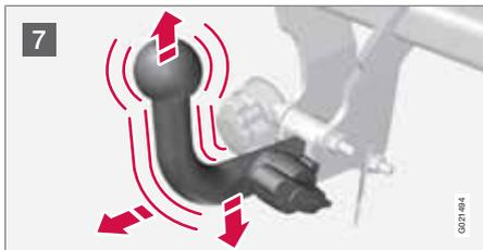
7 Check that the towbar is secure by pulling it up, down and back.
