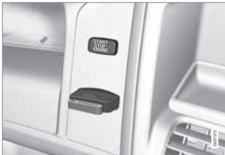
Ignition switch with inserted remote control key.
