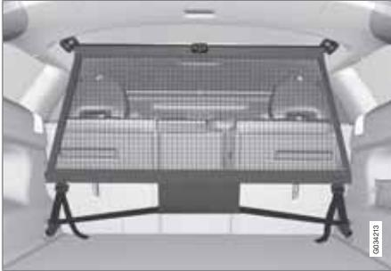
The safety net is fitted into four mounting points.
