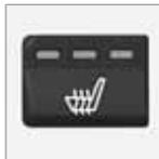
Press the button once for the highest heat level – three lamps illuminate.
