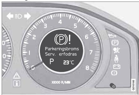
**Park brake not fully released** - A fault is preventing the parking brake from being released. Visit a workshop - an authorised Volvo workshop is recommended. A warning signal sounds if you pull away with this error message.
