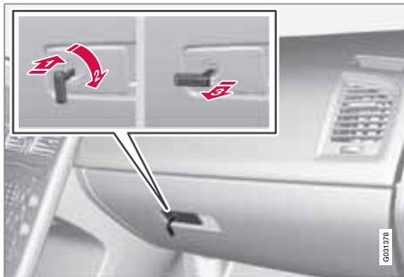
The glovebox can only be locked/unlocked using the remote control key's detachable key blade. (For information on the key blade, see page 49).
