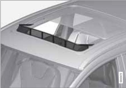
The panorama roof has a wind deflector that is folded up when the panorama roof is in the open position.
