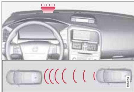
A small section of the red warning lamp in the windscreen illuminates with a constant glow if the distance to the vehicle in front is shorter than the set time interval.
