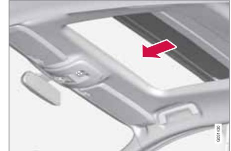
One long press on the lock button, see pages 47 (remote control key) and 56 (central locking button), closes the panorama roof and all the windows. The door mirrors are retracted\* and the doors and tailgate are locked. To interrupt closing, press the lock button again.
