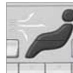
The figure consists of three buttons. When the buttons are pressed a lamp in front of the respective part of the figure illuminates and shows which air distribution is selected, see page 141.
