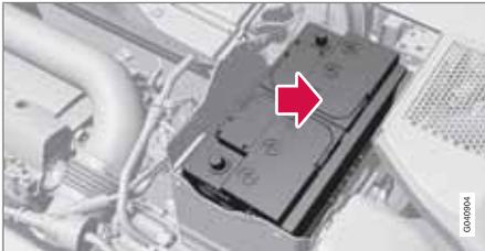
1. Lower the battery into the battery box.
