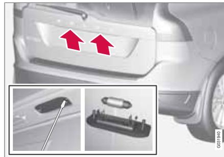
1. Remove the screws with a screwdriver.
