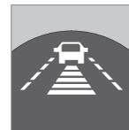
Different time intervals to the vehicle in front can be selected and shown in the display as 1-5 horizontal lines - the more lines the longer the time distance. One line corresponds to approximately
