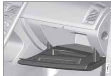
The owner's manual and maps can be kept here for example. There are also holders for pens on the inside of the lid. The glovebox can be locked with the key blade, see page 49.
