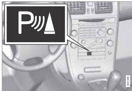
The system is automatically activated when the car is started and the switch's On/Off lamp is illuminated. If parking assistance is switched off with the button, the lamp goes out.
