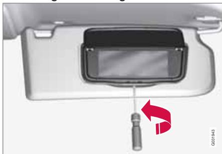
1. Insert a screwdriver underneath the lower edge, in the centre. Carefully prize up the lug on the edge.
