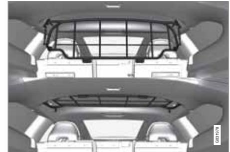
A safety grille prevents loads or pets from being thrown forward in the passenger compartment in the event of sudden braking.
