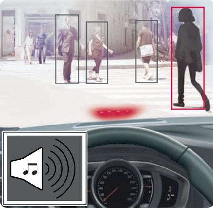
Collision Warning with Auto Brake and Cyclist and Pedestrian Detection, which can warn, brake and/or stop for vehicles, cyclists and pedestrians.
