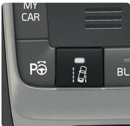
If the car is about to cross a side line the LKA will actively steer back into the lane with a slight steering torque in the steering wheel. If the car crosses a side line then LKA will warn you with pulsating vibration in the steering wheel.
