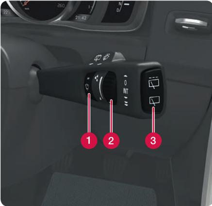
Move the lever downward to start the windscreen wipers and upward for a single sweep.
