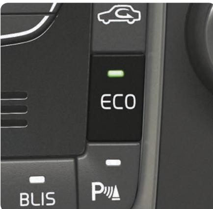
One press on **ECO** activates an optimal fuel-efficient driving program including, amongst other things, the following changes:
