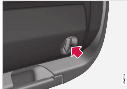
Lamp housing on left-hand side.
