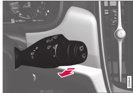
Washing function, right-hand stalk switch.
