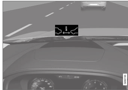
Symbol for Distance Warning on the windscreen 32 .
