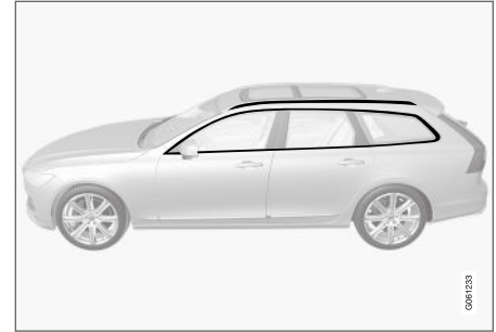
Parts that should be washed using a cleaning agent with a pH value between 3.5 and 11.5.
