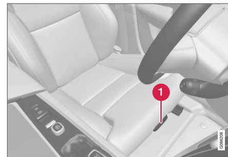
Control for seat cushion adjustment.
