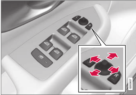
Controls for door mirrors.
