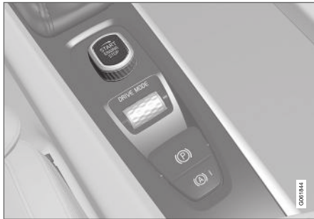
Start knob in the tunnel console.
