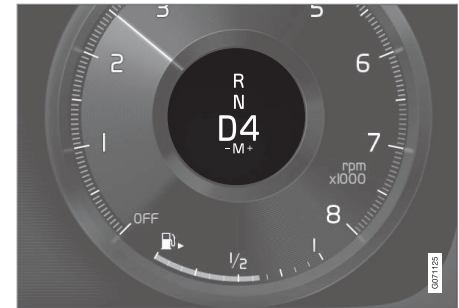
Driver display when changing gear with steering wheel paddles, small gear lever.
