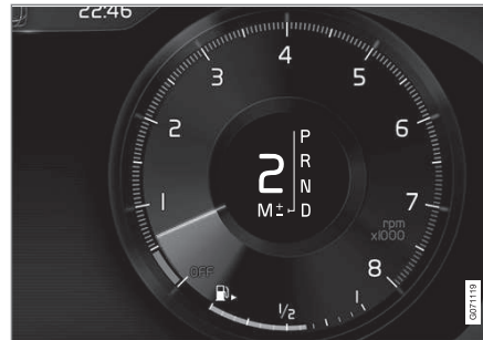
Overview of the shift pattern in the driver display for large gear lever.
