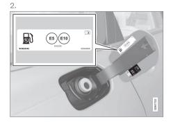
Choose fuel that is approved for use in the car in accordance with the identifier<sup>10</sup> on the inside of the fuel filler flap. See information on approved fuels and identifier in the section on "Petrol".
