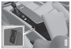
USB inputs (type A) in the tunnel console. Allow the cable to lie forwards so that it is not trapped when the lid is closed.
