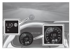
The previous illustration shows that Pilot Assist is set to maintain 110 km/h (68 mph) and that there is no vehicle ahead to follow.
