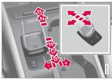
Overview of gear lever and gear positions.
