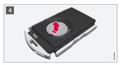
4 The battery (+) side is facing upwards. Then carefully prize loose the battery as illustrated.
