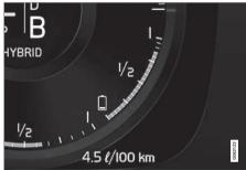
The energy in the hybrid battery is used for the electric motor, but also to cool or heat the car. The trip computer calculates an approximate distance for the energy left in the hybrid battery.
