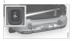
Open the boot lid. A button for extending/ retracting the towbar is located on the right-hand side at the rear of the cargo area. An indicator lamp in the button must illuminate with a constant orange glow for the extension function to be active.  Press and release the button – extension might not start if the button is pressed for too long.
