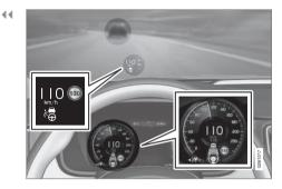
The previous illustration shows that Pilot Assist is set to maintain 110 km/h (68 mph) and at the same time is following a vehicle ahead which is keeping the same speed.
