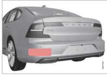
Keep the surface indicated clean – on both the left and right-hand sides of the  $car^{86}$ .
