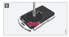
Refit the battery cover and turn it clockwise until the marking aligns with the **CLOSE** text.
