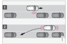
Principle for reversing into parallel parking.
