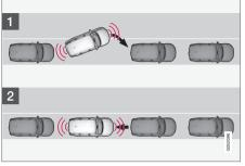
Principle for positioning during parallel parking.
