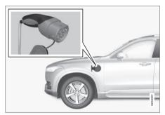
Charging cable handle and charging input socket.
