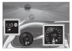
The previous illustration shows that the adaptive cruise control is set to maintain 110 km/h (68 mph) and at the same time is following a vehicle ahead which is keeping the same speed.
