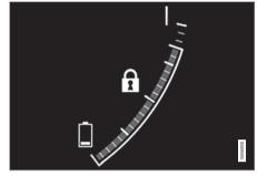
The ft symbol in the hybrid battery gauge indicates that the Hold function is activated, and the **f** symbol indicates that the Charge function is activated.
