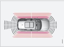
The warning signal pulses intensively at less than approx. 25 cm (0.8 ft) from an obstacle.
