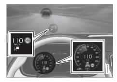
The previous illustration shows that Pilot Assist is set to maintain 110 km/h (68 mph) and at the same time is following a vehicle ahead which is keeping the same speed.
