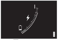
The symbol **5** is shown in the hybrid battery gauge when Charge is activated.
