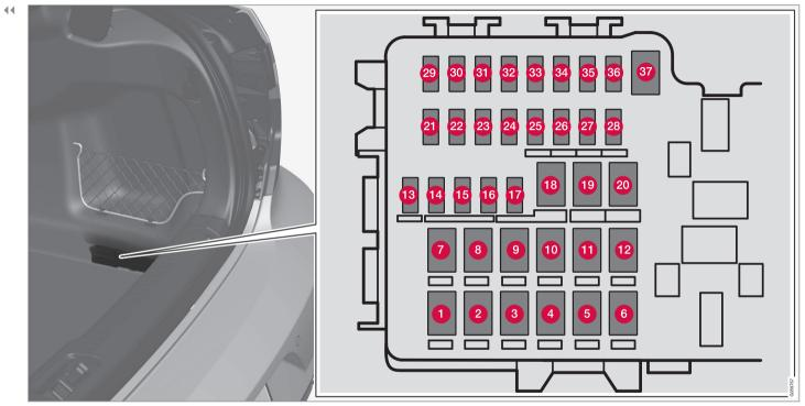
The central electrical unit is located on the right-hand side.
