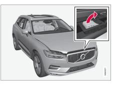
Sweep from left to right in the opening under the bonnet, move the handle up and to the side to release the bonnet from the bonnet lock's catch and lift the bonnet.
