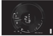
The car generates current to the battery and the battery is charged, e.g. when the brake pedal is pressed gently or during engine braking down a hill.
