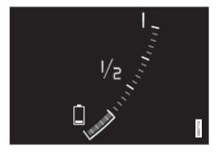
If the state of charge is high – run the car until approx. 25% remains. If the state of charge is low – charge the battery until a level of approx. 25% is reached.  If storage has lasted longer than 6 months or the hybrid battery charge level is significantly lower than 25% – charge the battery to approx. 25% again to compensate for the natural self-discharge that occurred during the prolonged storage. Continuously check the charge level in the driver display.
