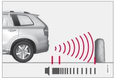
The warning signal has a constant tone at less than approx. 30 cm (1 ft) from an obstacle.
