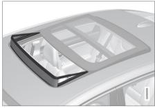
The panorama roof has a wind deflector that is raised when the panorama roof is in the open position.
