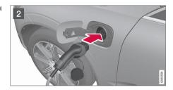
Open the charging hatch. Remove the charging handle's protective cover and then press the handle the whole way into the socket for the car.
