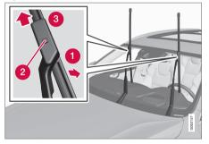
Fold up the wiper arm when it is in service position. Service position is activated/deactivated via the function view in the centre display when the car is stationary and the windscreen wipers are not on.
