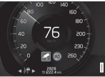
Examples of information on speed camera and speed limit in the driver display.
