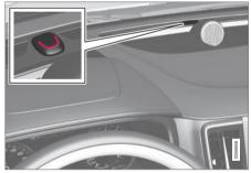
A red LED on the instrument panel flashes once every two seconds when the car is locked and the alarm is armed.
