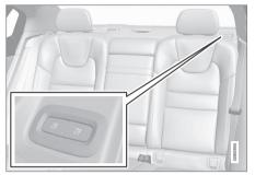
Buttons for seat folding, located on the upper section of the rear seat.
