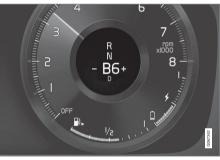
Gear shift indicator in the driver display<sup>5</sup>.
