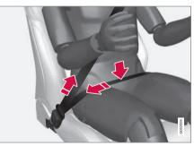
The hip strap must be positioned low down (not over the abdomen).
