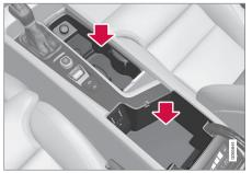
Storage spaces with cup holder, electrical socket and USB port in the tunnel console.
