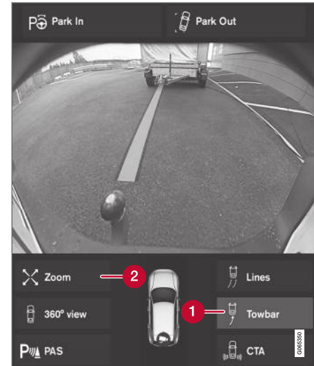
Towbar with trajectory line.
