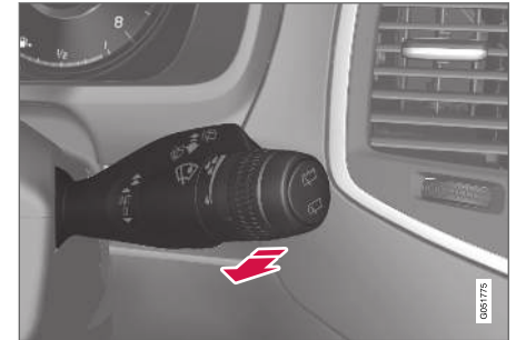
Washing function, right-hand steering wheel lever.
