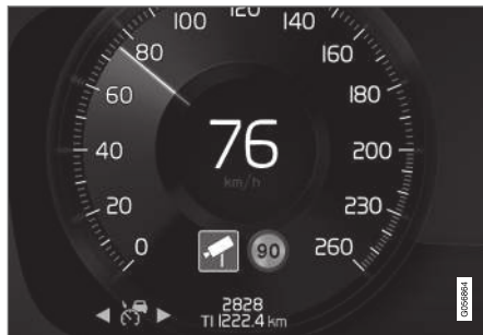
Speed camera information in the instrument panel.
