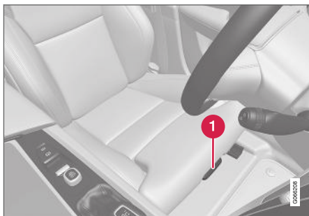
Control for adjusting seat cushion.
