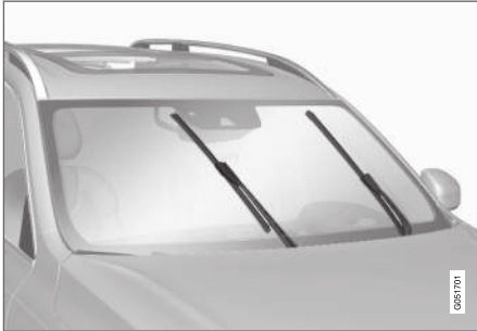
Windshield wipers in the service position.
