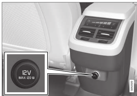
12 V outlet in the tunnel console, second row of seats.
