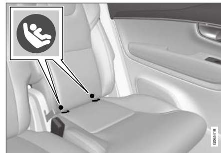
Location of the ISOFIX/LATCH anchors
