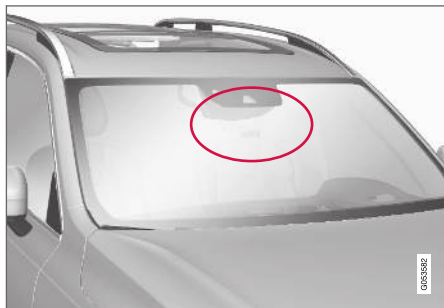
Location of radar sensor.
