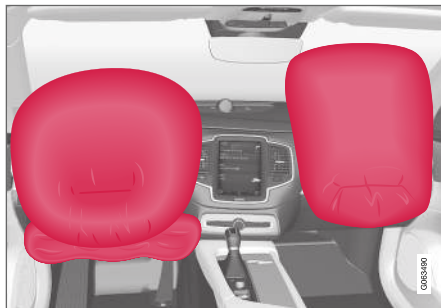
Driver/passenger side front airbags.
