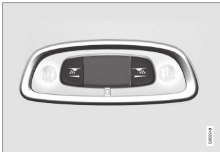
Reading lights over the rear seat 4 .
