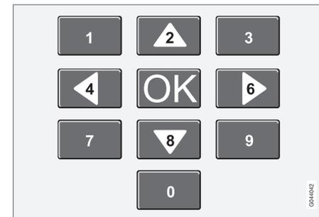
Navigation in the DVD video disc's menu is performed using the number keys in the centre console as illustrated above.
