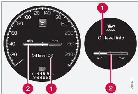
Message and graph in the display. The left-hand display shows the digital combined instrument panel and the right-hand the analogue.
