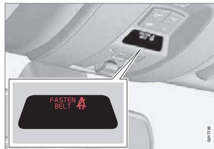
Unbelted occupants will be reminded to fasten their seatbelts by means of an audio and visual reminder. The audible reminder is speed dependent, and in some cases time dependent. The visual reminder is located in the roof console and in the combined instrument panel.
