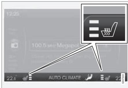
Current heat level is shown in the centre console's screen.
