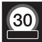
A symbol for additional sign in the form of an empty frame under the combined instrument panel's speed symbol means that the RSI has detected an additional sign with supplementary information for the current speed limit.
