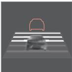
Different time intervals to the vehicle in front can be selected and shown in the combined instrument panel as 1-5 horizontal lines - the more lines the longer the time interval. One line corre-
