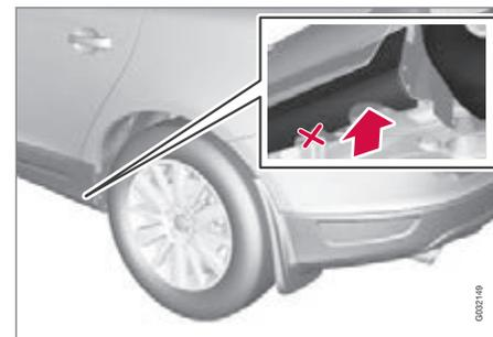
Check that the jack sits in the anchorage as illustrated and that the foot is positioned vertically under the anchorage.
