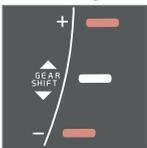
Gear shift indicator for manual gearbox. Only one marker is illuminated at a time - during normal driving it is only illuminated in the centre.
