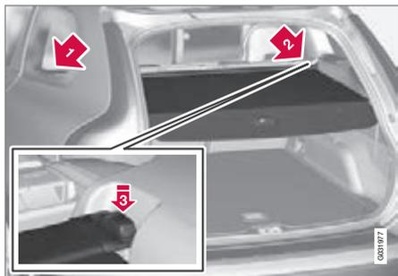
Pull the cargo cover over the load and hook it into the recesses at the cargo area's rear posts.
