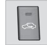
When recirculation is engaged the orange lamp in the button illuminates. The function is selected to shut out bad air, exhaust gases etc. from the passenger compartment. The air in the passenger compartment is recirculated, i.e. no outside air is taken into the car when this function is activated.
