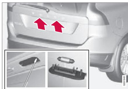
1. Remove the screws with a screwdriver.
