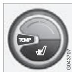
The temperature can be adjusted with the knob. For ECC\* the temperature for the driver's side and the passenger side can be set separately.
