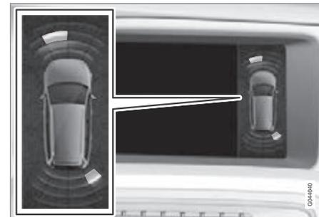
Screen view - showing an obstacle left front and right rear.
