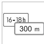
Some speeds are applicable only after e.g. a specific distance or at a certain time of day. The driver's attention is drawn to the situation by means of a symbol for an additional sign under the
