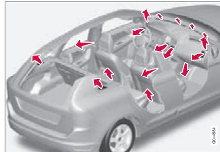
The incoming air is divided between a number of different vents in the passenger compartment.
