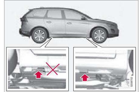
If the car is raised with a workshop jack; position the jack against the front edge on the engine's subframe.
