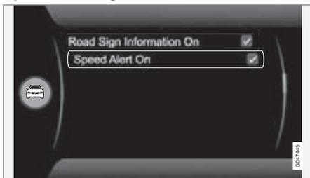
The driver can opt to receive a warning when the applicable speed limit is exceeded by 5 km/h or more. This warning is given by the symbol showing the applicable maximum speed temporarily flashing when this speed is exceeded.
