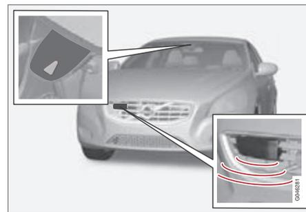
Camera and radar sensor<sup>3</sup>.
