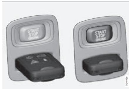
2. Insert the remote control key in the ignition switch.
