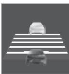
Only when the symbol shows the image of another vehicle is the **distance** to the vehicle ahead regulated by the cruise control.
