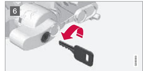
6 Turn the key anticlockwise to locked position. Remove the key from the lock.
