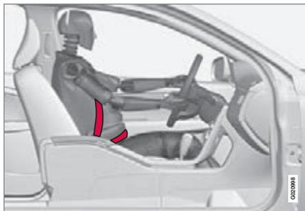
The seatbelt should always be worn during pregnancy. But it is crucial that it be worn in the correct way. The diagonal section should wrap over the shoulder then be routed between the breasts and to the side of the abdomen.
