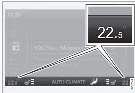
Current temperature for each side is shown in the centre console's screen.
