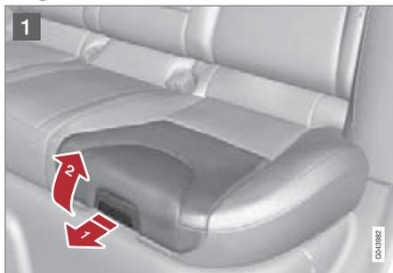
**1** Pull the handle forward and up in order to release the booster cushion.
