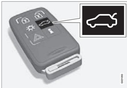
The alarm for the tailgate can be disarmed\* and the tailgate unlocked on its own by using the remote control key's
