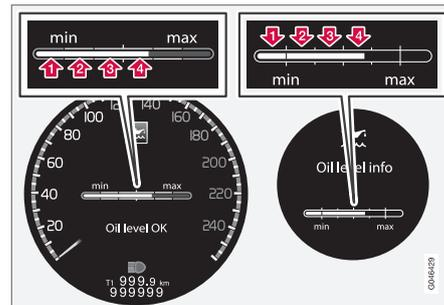
The figures 1-4 represent filling level. Do not fill more oil if filling level (3) or (4) is shown. Recommended filling level is 4. Message and graph in the display. The left-hand display shows the digital combined instrument panel and the right-hand the analogue.
