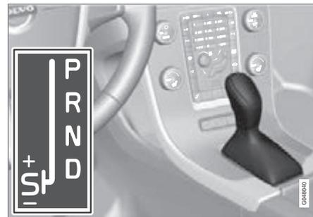
D: Automatic gear positions. +/-: Manual gear positions. S: Sport mode\*.
