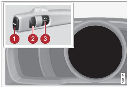
Information display (digital combined instrument panel) and controls for menu navigation.
