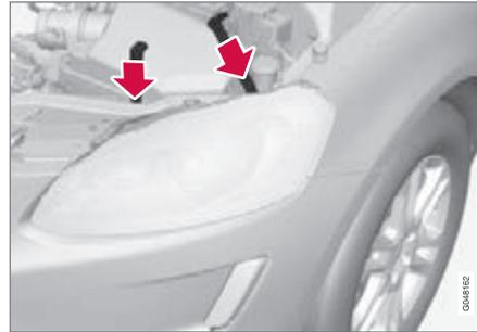
When securing, check that the long lock pin is engaged - it should be engaged in both eyes.
