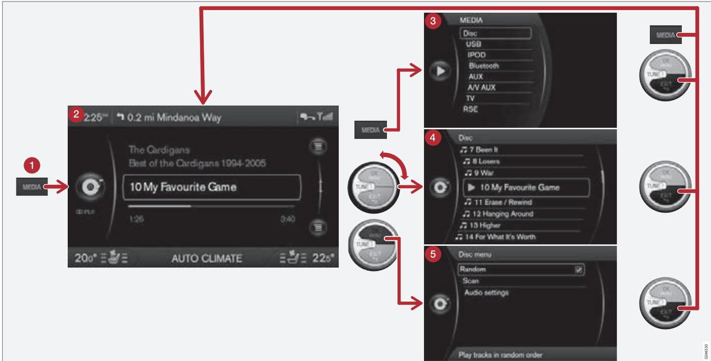
The example shows navigation to different functions when a disc is played back. (1) Main source button, (2) Normal view, (3) Shortcut/Source menu, (4) Quick menu, (5) Source menu.
