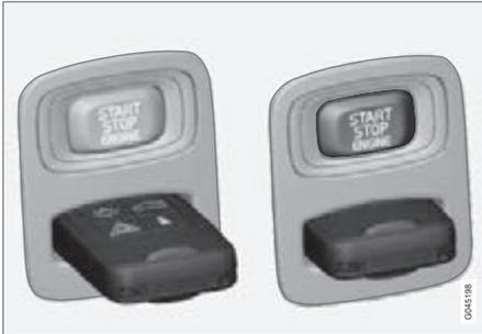
Ignition switch with remote control key extracted/inserted.
