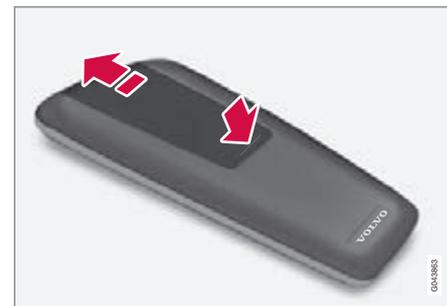
1. Push down the catch on the battery cover and slide the battery cover in the direction of the infrared lens.
