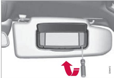
1. Insert a screwdriver under the lamp lens and gently prize up the lock lugs on the edge.
