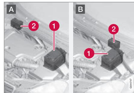
A: Left-hand drive car. B: Right-hand drive car. 1. Battery for starting<sup>3</sup> 2. Support battery.
