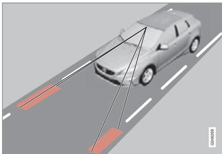
The LDW (Lane Departure Warning) function is intended to reduce the risk of so-called single-vehicle accidents – accidents where, in certain situations, the vehicle leaves the carriageway and is in danger of driving either into a ditch or into oncoming traffic.
