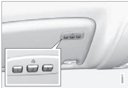
HomeLink®<sup>1</sup> is a programmable remote control which can remotely control up to three different devices (e.g. garage door opener, alarm system, outdoor lighting and indoor lighting etc.) and in doing so replace their remote controls. For more information on HomeLink®, visit: [www.homelink.com](http://www.homelink.com) or ring 00 8000 466 354 65 (or premium rate phone number, +49 6838 907 277).
