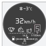
With "Analogue" combined instrument panel, the gear positions and indicator arrows are displayed in its centre.
