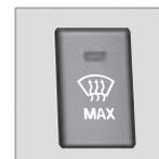
Used to quickly remove misting and ice from the windscreen and side windows. The light in the defroster button illuminates when the function is active.
