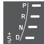
Automatic gear positions are indicated on the right of the combined instrument panel. (Only one marker is illuminated at a time - the one showing the current gear selector position.)
