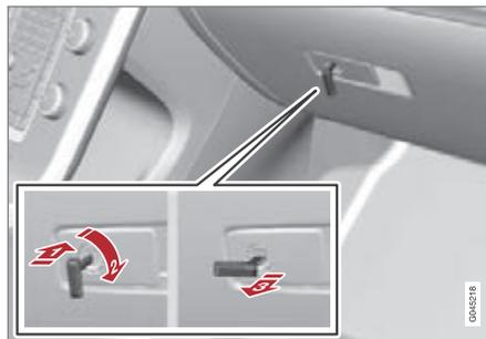
The glovebox can only be locked/unlocked using the remote control key's detachable key blade. For information on the key blade, see page 50.
