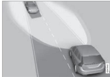
*Dipped beam directly toward oncoming vehicles, but continued main beam on both sides of the vehicle.*
