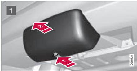
1 Remove the protective cover by first pressing in the catch
