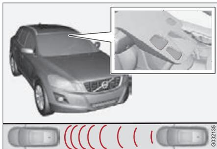
Laser sensor transmitter and receiver window<sup>1</sup>.
