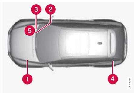
Central electrical unit locations in a left-hand drive car. In a right-hand drive car the central electrical units under the glovebox change sides.
