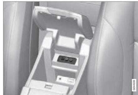
*The A/V-AUX input is located under the armrest in the tunnel console.*
