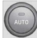
The Auto function automatically regulates temperature, air conditioning, fan speed, recirculation, and air distribution.
