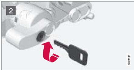
2 Ensure that the mechanism is in the unlocked position by turning the key clockwise.
