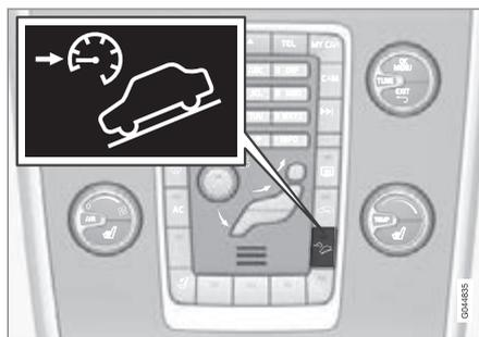
HDC is engaged or disengaged using a switch on the centre console. An indicator lamp in the button illuminates when the function is switched on.
