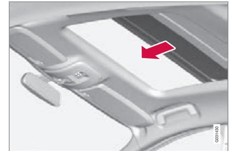
One long press on the lock button, see pages 47 (remote control key) and 57 (central locking button), closes the panorama roof and all the windows. The door mirrors are retracted\* and the doors and tailgate are locked. To interrupt closing, press the lock button again.
