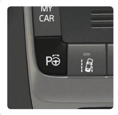
PAP checks the available space, and then steers in the car. Your task is to keep a close watch around the car, change gear, control the speed and brake/stop.
