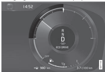
Eco gauge in the 12-inch driver display*.
