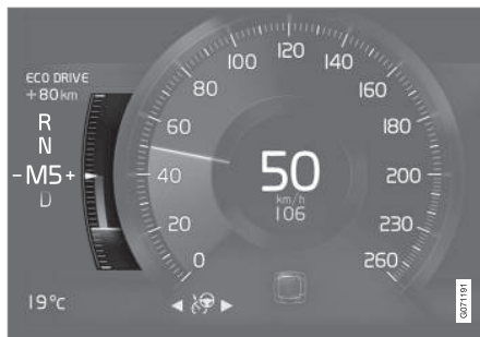
Eco gauge in the 8-inch driver display.
