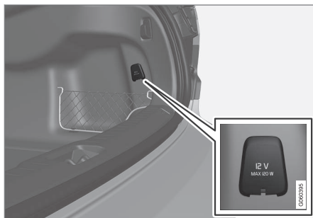
12 V electrical socket in cargo area*.
