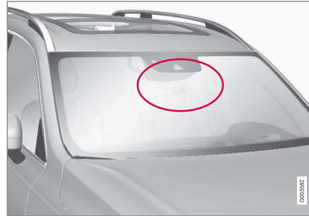
Radar unit location.
