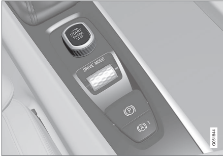
Start knob in the tunnel console.
