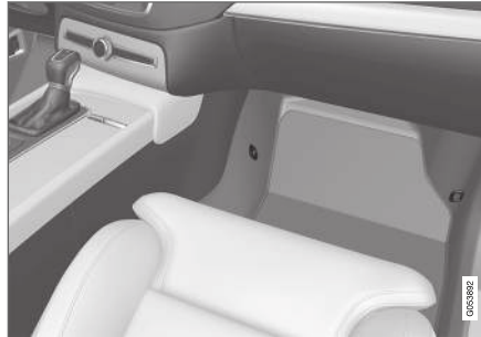
Mounting point locations in the front seat.
