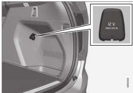
12 V electrical socket in cargo area*.
