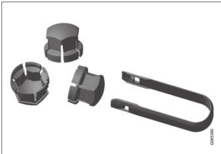
Tool for removing the plastic covers on the wheel bolts.
