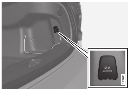
12 V outlet in trunk/cargo compartment*.
