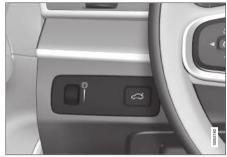
Thumbwheel (to left) for adjusting interior brightness.
