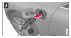
Open the charging hatch. Remove the charging handle's protective cover and then press the handle the whole way into the socket for the car.
