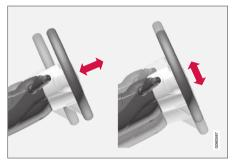
The steering wheel can be adjusted for height and for depth.
