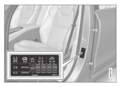
The decal displays the designation for the factory-fitted tyres on the car, as well as load limits and tyre pressure.
