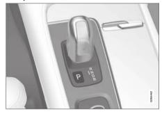
The park position is activated via the **P** button next to the gear selector.
