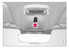
The sunroof is operated with a control located in the roof. The control is activated when the car's electrical system is in ignition position  ${\bf I}$  or  ${\bf II}$ .
