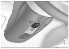
Lever for steering wheel adjustment.
