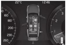
Graphics in the driver display with different types of warnings. The warning colour on the door and boot lid is dependent on the speed of the car.
