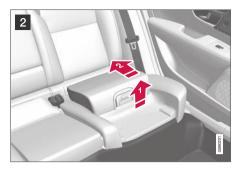
Lift the seat cushion up at the front edge and press it back against the backrest to lock.
