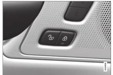
Locking and unlocking button with indicator lamp in the front door.
