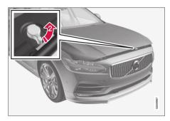
Turn the handle under the bonnet anticlockwise to release the bonnet from the lock catches and lift the bonnet.
