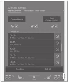
Functions belonging to the parking climate control are controlled from the **Parking climate** in climate view in the centre display.
