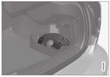
The charging cable is located in the storage compartment to the right of the cargo area.
