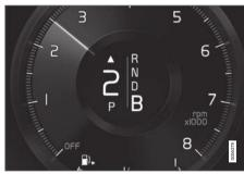
Gear shift indicator in the driver display<sup>3</sup>.
