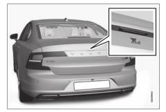
Rubberised pressure plate on the boot lid used for unlocking only.
