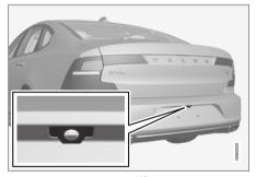
The backwards-facing camera  $^{\!115}\!$  is fitted above the registration plate.
