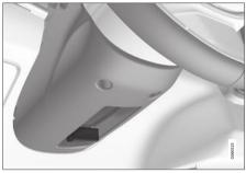
Lever for steering wheel adjustment.
