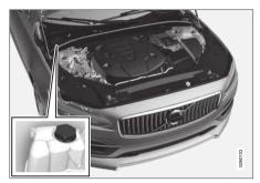
Coolant expansion tank, left-hand drive car.
