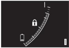
The symbol in the hybrid battery gauge indicates that the **Hold** function is activated, and the symbol indicates that the **Charge** function is activated.
