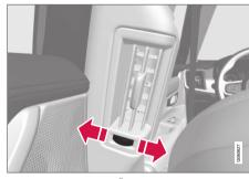
The air vent's thumbwheel<sup>2</sup>.
