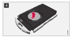
The battery (+) side is facing upwards. Then carefully prize loose the battery as illustrated.
