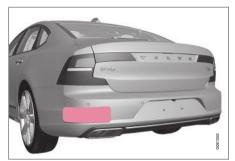
Keep the surface indicated clean – on both the left and right-hand sides of the car<sup>77</sup>.
