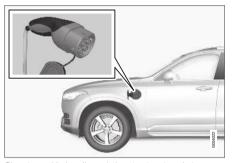
Charging cable handle and charging input socket.
