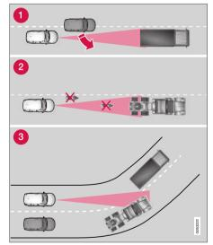
The radar sensor's field of vision.
