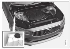
Coolant expansion tank, left-hand drive vehicle.
