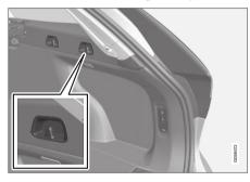
There are two grocery bag holders in the side panel on each side of the cargo compartment.
