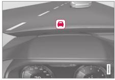
Collision warning symbol on the windshield<sup>70</sup>.
