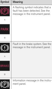
A flashing symbol indicates that a fault has been detected. See the message in the instrument panel.
