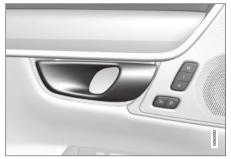
Alternative unlocking method using side door opening handle  $^{15}\!\!\!\!$
