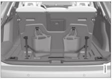
There are two grocery bag holders and an elastic  $band^3$  in the hatch in the cargo compartment floor. The strap can be attached in four different positions.
