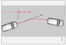
Lane Keeping Aid alerts the driver using vibrations in the steering wheel<sup>103</sup>.
