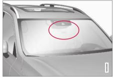
The area marked in the illustration must be kept free of decals, objects, solar film, etc.  $^{63}$
