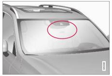
The area marked in the illustration must be kept free of decals, objects, solar film, etc.  $^{67}$
