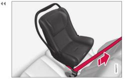
Pull out the shoulder section of the seat belt.
