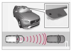
Location of the camera and radar sensor<sup>68</sup>.
