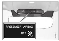
Occupant Weight Sensor (OWS) indicator light
