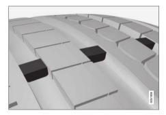
The tread wear indicator is a narrow elevated strip running across the tire's longitudinal tread grooves. The letters TWI (Tread Wear Indicator) are visible on the side of the tire. When approximately 1.6 mm (1/16 inch) is left on the tread, the tread will be at the same height as the tread wear indicator. Replace the tire as soon as possible. Tires with low tread offer very poor traction in rain or snow.
