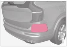
Keep the marked area clean (on both the left and right sides of the vehicle)<sup>77</sup>.
