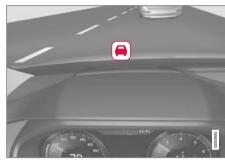
Collision warning symbol on the windshield<sup>57</sup>.
