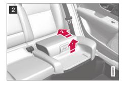
2 Lift the front edge of the booster cushion and press it rearward toward the backrest to lock it into position.
