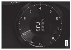
Manual shifting mode in the instrument panel<sup>2</sup>.
