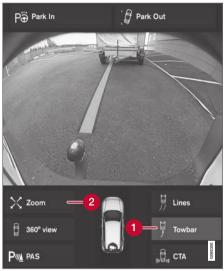
Towbar with trajectory line<sup>117</sup>.
