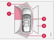
Parking sensor sectors where obstacles can be detected<sup>118</sup>.
