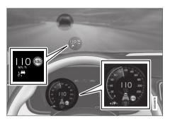
The previous illustration<sup>62</sup> shows that Pilot Assist is set to maintain a speed of 110 km/h (68 mph) and is following a target vehicle ahead that is traveling at the same speed.
