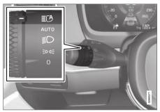
Active high beam is enabled by moving the lighting ring on the steering wheel lever to  $\ensuremath{\,\text{AUT0}}$  .
