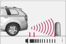
Continuous tone warning signal when the obstacle is less than approx. 30 cm (1 ft) from the vehicle  $^{110}\,$
