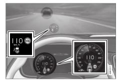
The previous illustration<sup>62</sup> shows that Pilot Assist is set to maintain a speed of 110 km/h (68 mph) and is following a target vehicle ahead that is traveling at the same speed.
