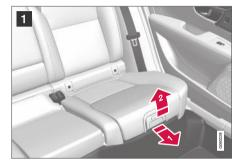
Pull the handle forward and upward to release the booster cushion.
