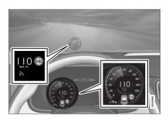
The previous illustration<sup>54</sup> shows that Adaptive Cruise Control is set to maintain a speed of 110 km/h (68 mph) and that there is no target vehicle ahead to follow.
