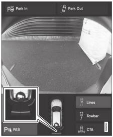
The screen can display colored sensor fields on the vehicle symbol<sup>118</sup>.
