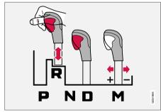
The gear selector can be moved back and forth between  ${\bf N}$  and  ${\bf D}$ . The other positions have a shiftlock that is operated using the lock button on the gear selector.
