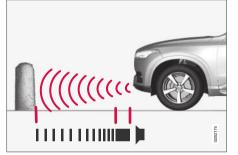
Continuous tone warning signal when the obstacle is less than approx. 30 cm (1 ft) from the vehicle  $^{110}\!\!.$
