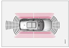
Rapid pulsing warning signal when the obstacle is less than approx. 25 cm (0.8 ft) from the vehicle  $^{110}$ .
