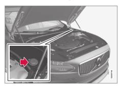
Fill washer fluid into the reservoir with the blue cover. The reservoir is used for the windshield washer, tailgate window washer and headlight washer\*
