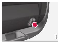
1. Remove the panel on the inside of the tailgate by turning both clips counterclockwise a quarter-turn. Remove the panel. Place the panel in a safe location out of the way.
