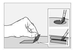
1. Place a strip of masking tape over the damaged surface. Pull the tape off so that any loose flakes of paint adhere to it.
