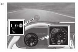
The previous illustration  $^{62}$  shows that Pilot Assist is set to maintain a speed of 110 km/h (68 mph) and that there is no target vehicle ahead to follow.
