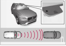
The camera/radar sensor measures the distance to the vehicle ahead  $^{\rm 37}\!.$
