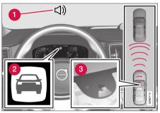
Collision warning audible signal and symbol<sup>56</sup>.
