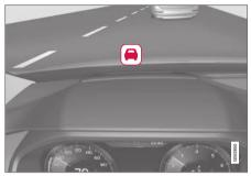
Collision warning symbol on the windshield<sup>39</sup>.
