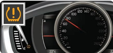
Calibration is always required after changing tyres or changed tyre pressure. In the event of lamp illumination (⚠) the tyre pressure needs to be checked and the system calibrated. Proceed as follows:
