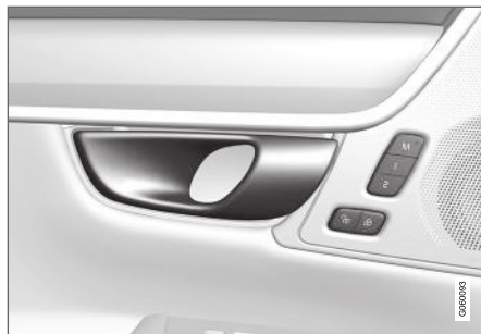
Opening handle for alternative unlocking in the side door 15 .
