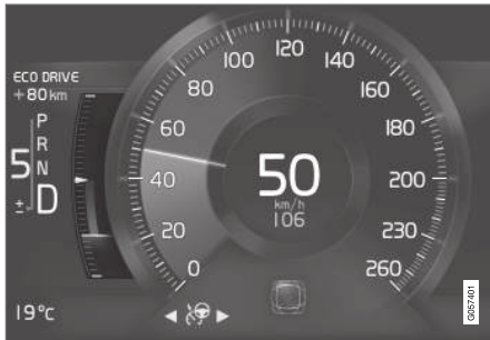
Eco gauge in the 8-inch driver display.
