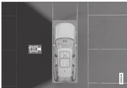
The car's left-hand camera is out of order.
