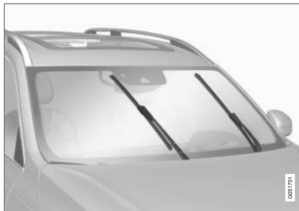
Wiper blades in service position.
