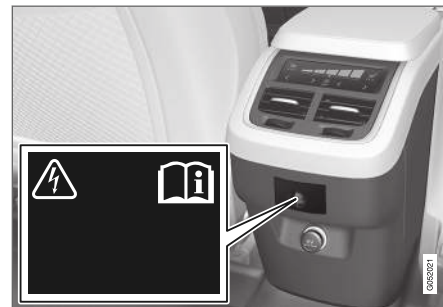
Electrical socket in the tunnel console, second seat row.
