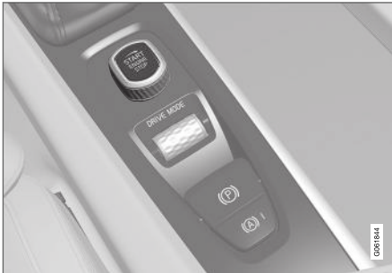
Start knob in the tunnel console.
