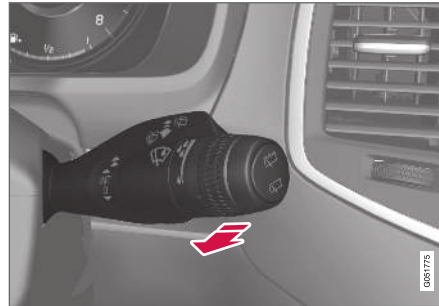
Washing function, right-hand stalk switch.
