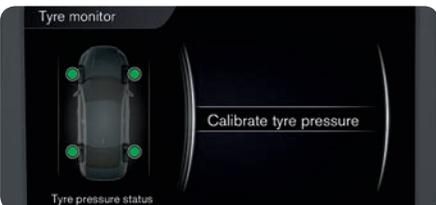
Calibration is always required after changing tyres or changed tyre pressure. In the event of lamp illumination (⚠) the system needs to be calibrated. Proceed as follows:
