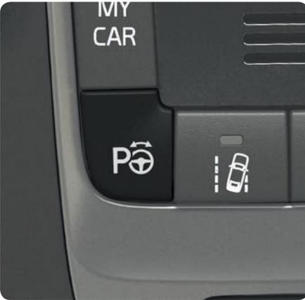
PAP checks the available space, and then steers in the car. Your task is to select the gear, control the speed and brake/stop.
