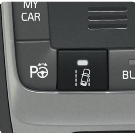
If the car is about to cross a side line the LKA will actively steer back into the lane with a slight steering torque in the steering wheel. If the car crosses a side line then LKA will warn you with pulsating vibration in the steering wheel.
