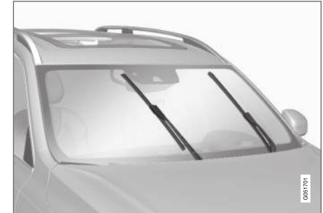
Viskerblader i servicestilling.
