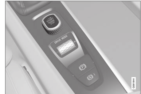
Start knob in the tunnel console.
