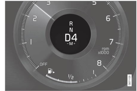
Instrument panel when shifting gears using steering wheel paddles, small gear selector.
