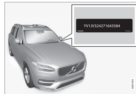
The VIN has a similar location on all models.
