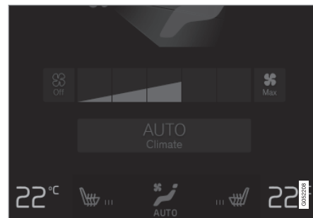
Temperature buttons in the climate bar.
