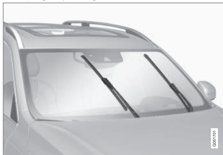
Windshield wipers in the service position.
