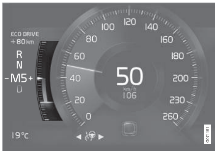
Eco gauge in 8" instrument panel.
