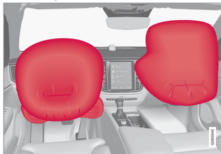
Driver/passenger side front airbags.
