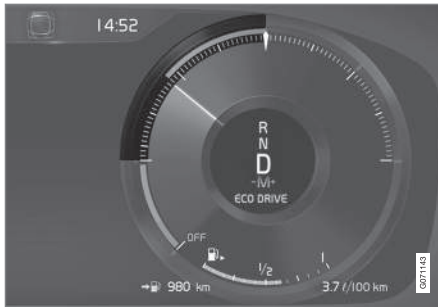
Eco gauge in 12" instrument panel*.
