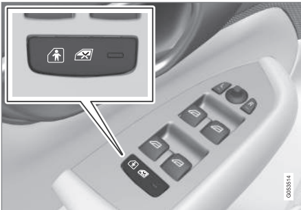
Button for electric activation and deactivation.
