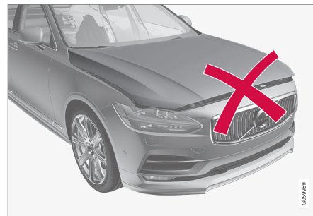
Hood not completely closed.
