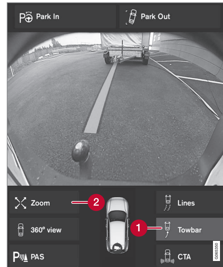
Towbar with trajectory line.
