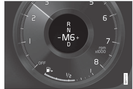
Overview of gear shift pattern in the instrument panel for small gear selector.
