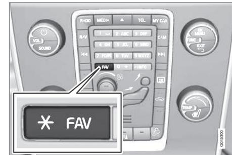
**FAV**The button can be used to save functions that are used frequently so that the function can be started simply by pressing **FAV**. You can select a favourite (e.g. **Equalizer**) for each function in accordance with the following:
