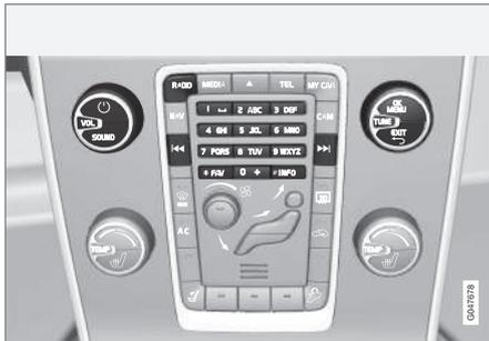
Controls for radio functions.
