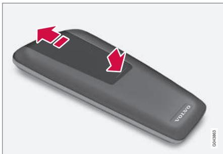
1. Push down the catch on the battery cover and slide the battery cover in the direction of the infrared lens.
