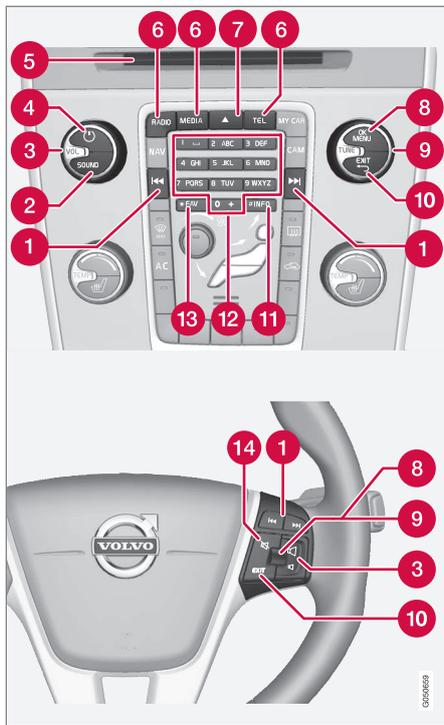
**1** Scroll/fast wind/search - Short press scrolls between disc tracks, preset radio stations<sup>1</sup> or chapter<sup>2</sup>. A long press fast
