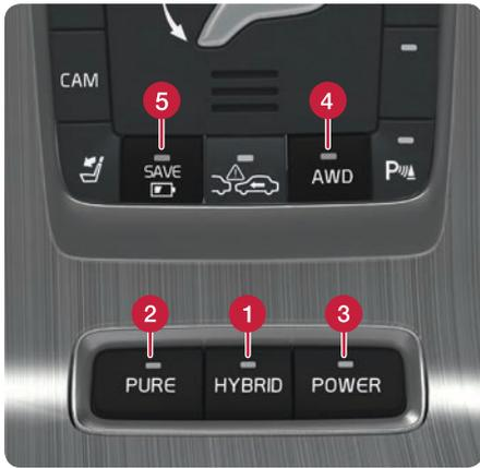
The car is powered by two motors - an electric motor and a diesel engine. Different drive modes can be selected. It is not possible to select the "wrong" drive mode - the car returns to the HYBRID mode if certain conditions are not met. The lamp in the hybrid button will then illuminate.
