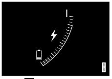
The symbol **y** is shown in the hybrid battery gauge when Charge is activated.
