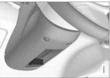
Lever for steering wheel adjustment.
