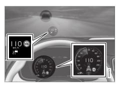
The previous illustration<sup>50</sup> shows that Pilot Assist is set to maintain 110 km/h (68 mph) and at the same time is following a vehicle ahead which is keeping the same speed.
