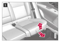
Pull the handle forwards and upwards to release the seat cushion.
