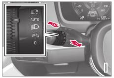
Steering wheel stalk switch with rotating ring.
