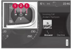
Examples of messages in the driver display and the steering wheel's right-hand keypad.
