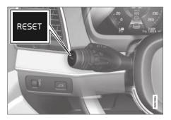
Reset all information in trip meter TM (i.e. mileage, average consumption, average speed and driving time) with a long press on the **RESET** button on the left-hand stalk switch.
