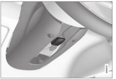
Lever for steering wheel adjustment.
