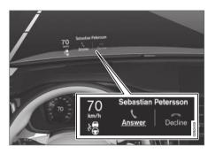
The head-up display shows warnings and information relating to speed, cruise control functions, navigation, etc. in the driver's field of vision. Road Sign Information and incoming phone calls can also be shown in the head up display.
