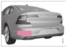
Keep the surface indicated clean – on both the left and right-hand sides of the  $car^{74}$ .
