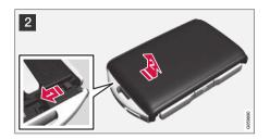
2 **1)** Turn the key, move the button to the side and slide the back shell a few millimetres upwards.
