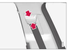
Press together the seat mounting and move the seatbelt up or down.
