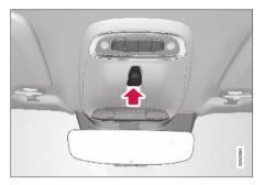
The sunroof is operated with a control located in the roof. The control is activated when the car's electrical system is in ignition position I or II.
