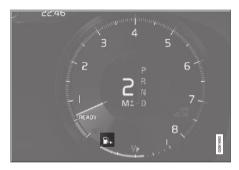
The beige zone in the fuel gauge indicates the quantity of fuel in the tank.
