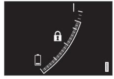
The f symbol in the hybrid battery gauge indicates that the Hold function is activated, and the symbol indicates that the Charge function is activated.
