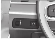
Thumbwheel (to left) for adjusting interior brightness.
