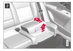
2 Lift the seat cushion up at the front edge and press it back against the backrest to lock.
