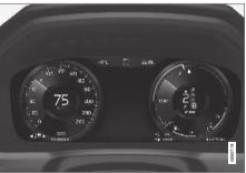
The driver display shows information on speed and e.g. incoming calls or song tracks being played. The display is operated via the two steering wheel keypads.
