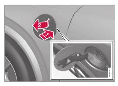
Press in the rear section of the cover and release.
