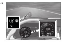
The previous illustration  $^{50}$  shows that Pilot Assist is set to maintain 110 km/h (68 mph) and that there is no vehicle ahead to follow.
