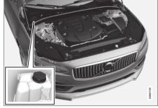
Coolant expansion tank, left-hand drive car.
