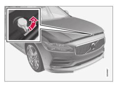
Turn the handle under the bonnet anticlockwise to release the bonnet from the lock catches and lift the bonnet.
