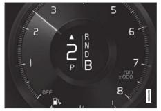
Gear shift indicator in the driver display<sup>5</sup>.
