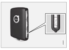
Long press on the remote control key's button. Keep it depressed until the boot lid starts to open.
