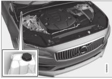
Coolant expansion tank, right-hand drive car.
