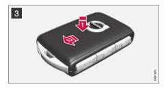
Return the key blade to its intended position in the remote control key after use.
