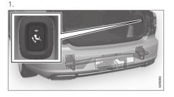
Open the boot lid. A button for extending/ retracting the towbar is located on the righthand side at the rear of the cargo area. An indicator lamp in the button must illuminate with a constant orange glow for the extension function to be active. 2. Press and release the button – extension might not start if the button is pressed for too long.
