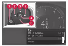
Open and navigate in the app menu<sup>2</sup> using the righthand steering wheel keypad.
