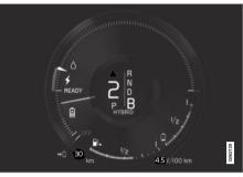
The car generates current to the battery, the battery is charged, e.g. when the brake pedal is pressed lightly or during engine braking down a hill.
