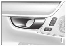
Opening handle for alternative unlocking in the side door<sup>12</sup>.
