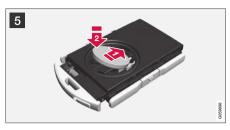
Install a new battery with the (+) side up.
