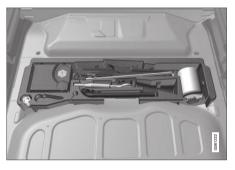
The foam block under the cargo area floor contains the car's towing eye, puncture repair kit, tool for removing the plastic caps from the wheel bolts and a socket for the lockable wheel bolts.
