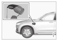
Charging cable handle and charging input socket.
