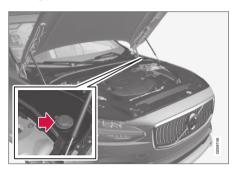
Washer fluid is filled into the reservoir with the blue cap. The reservoir is used for both wind-screen washer and headlamp washers\*
