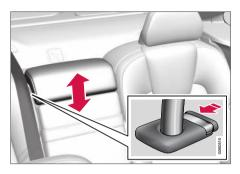
To lower the head restraint, the button (see illustration) must be depressed while the restraint is carefully moved down.
