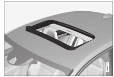
The sunroof has a wind deflector that is folded up when the sunroof is in the open position.
