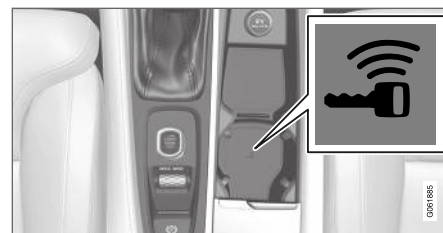
Backup reader's location in the tunnel console.
