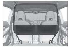
The cargo net is fitted into four mounting points.
