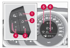
The steering wheel buttons and display in cars with speed limiter4.
