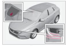
Camera and radar sensor<sup>24</sup>.
