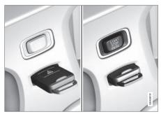
Ignition switch with remote control key extracted/inserted.
