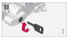
Ensure that the mechanism is in the unlocked position by turning the key clockwise.
