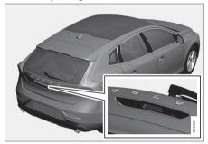
Rubber plate with electrical contact.
