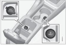
12 V socket in tunnel console, front seat,
