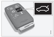
Using the remote control key (p. 160) button the alarm for the tailgate can be disarmed\* and the tailgate unlocked on its own.
