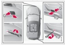
1. Take out the towing eye that is stored in the foam block under the cargo area floor.
