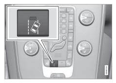
Press the centre console's button to activate or deactivate the function. The button's lamp illuminates when the function is switched on.
