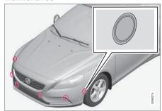
The PAP sensors are located in the bumpers<sup>40</sup> - 6 front and 4 rear.
