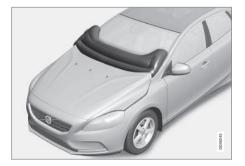
The pedestrian airbag (Pedestrian Airbag) is fitted under the bonnet near the windscreen. In the event of certain frontal collisions with a pedestrian, the sensors in the front bumper react and the airbag inflates if required, based on the force of the impact. The sensors are active at a speed of approx. 20-50 km/h (12-30 mph) and an ambient temperature between -20 and +70°C.
