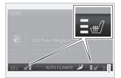
Current heat level is shown in the centre console display screen.
