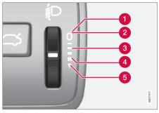
Thumbwheel positions for different load cases.
