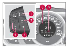
The steering wheel buttons and display in cars  $\mbox{\it with}$  speed limiter  $\!\!\!\!^7.$
