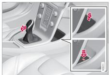
If the car cannot be driven, e.g. due to a flat battery, the gear selector must be moved from the **P** position so that the car can be moved.
