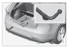
The detachable towbar must be stored in the foam block<sup>17</sup> under the cargo area floor when not in use.
