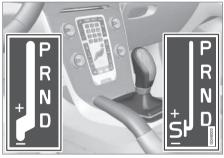
**D**: Automatic gear positions. +/-: Manual gear positions. **S**: Sport mode\*.3
