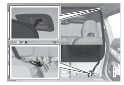
Hook the hooks into the roof mounting with the anchoring strap locks turned towards you.
