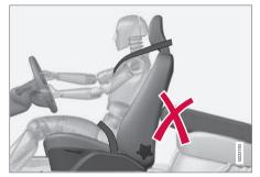
Do not place objects on the rear seat that may prevent the WHIPS system from functioning.
