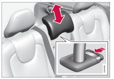
Adjust the head restraint according to passenger height so that the whole of the back of the head is covered if possible. Slide it up as required.
