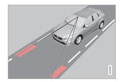
A camera reads the painted side lines of the road/lane. If the car is about to cross a side line then Lane Keeping Aid will actively steer the car back into the lane with a slight steering torque in the steering wheel.
