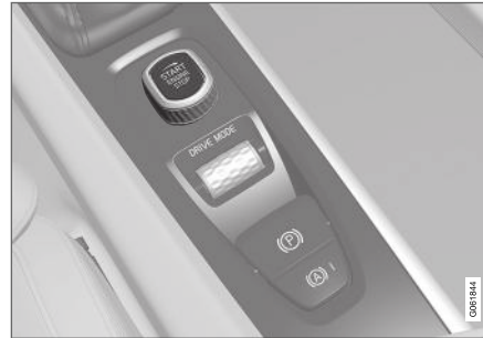
Start knob in the tunnel console.
