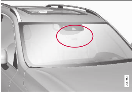
Location of radar sensor.
