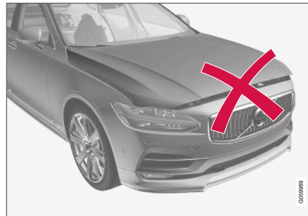
Hood not completely closed.
