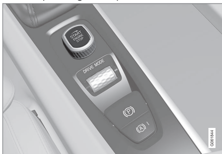
Start knob in the tunnel console.
