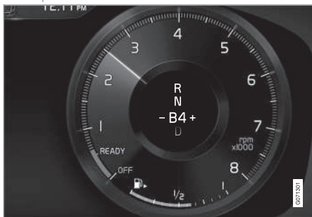
Driver display when changing gear with steering wheel paddles in manual gearshift mode.
