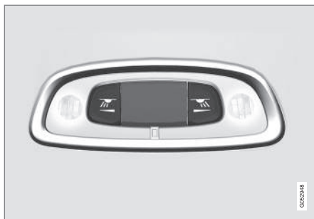
Reading lamps above the rear seat 6 .
