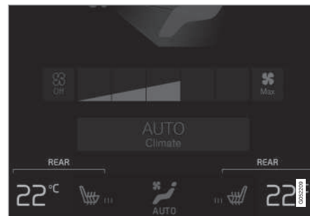
Temperature buttons in the Rear climate tab in the climate view.
