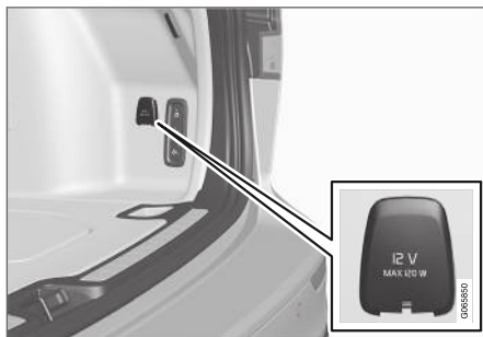
12 V outlet in trunk/cargo compartment*.
