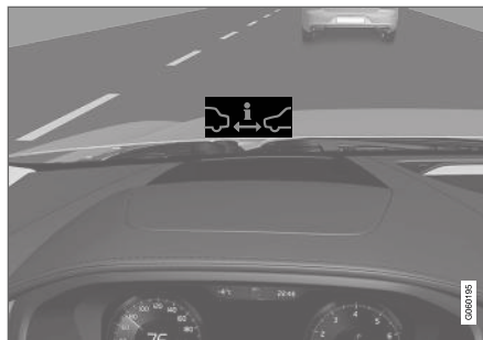
Distance Alert warning symbol on the windshield 36 .
