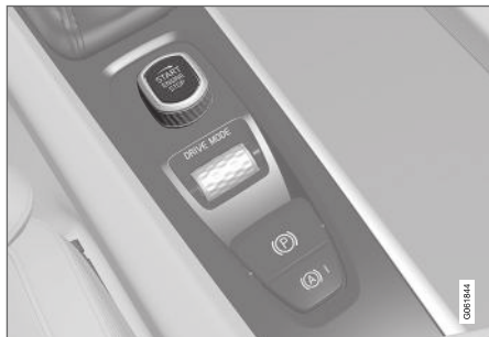
Start knob in the tunnel console.
