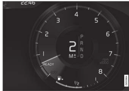
Manual shifting mode in the instrument panel 2 .
