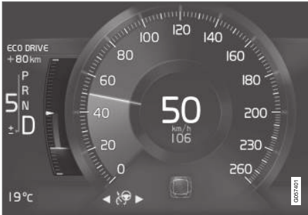
Eco gauge in 8" instrument panel.
