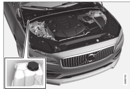
Coolant expansion tank, left-hand drive vehicle.
