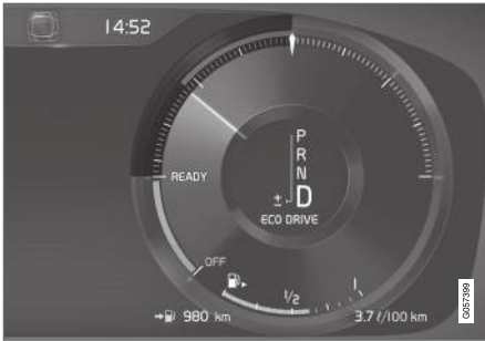
Eco gauge in 12" instrument panel*.
