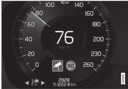
Speed camera information in the instrument panel 102 .
