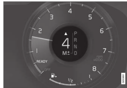
Gear indicator in 12" instrument panel*.
