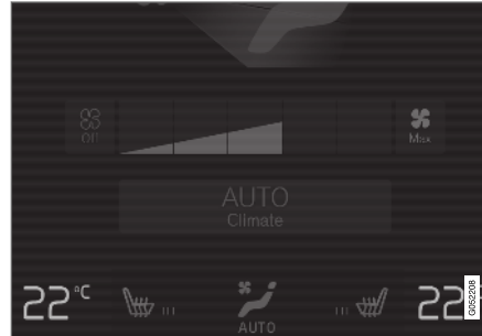
Temperature buttons in the climate bar.
