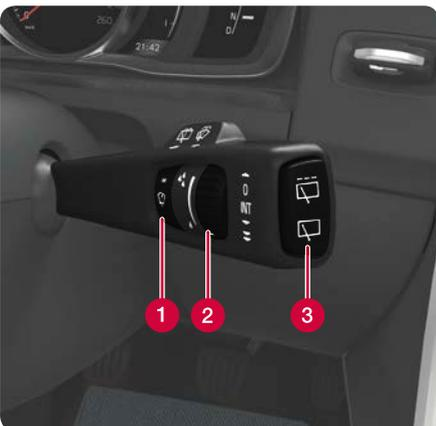
Move the lever downward to start the windscreen wipers and upward for a single sweep.
