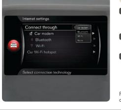
Connect the mobile phone via Bluetooth<sup>®</sup> or activate tethering in the phone for Wi-Fi connection. For car modem connection, fit the SIM card into the reader in the glovebox.
