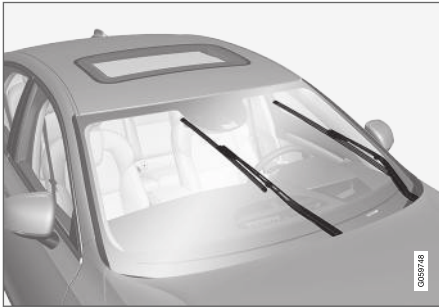
Viskerblader i servicestilling.
