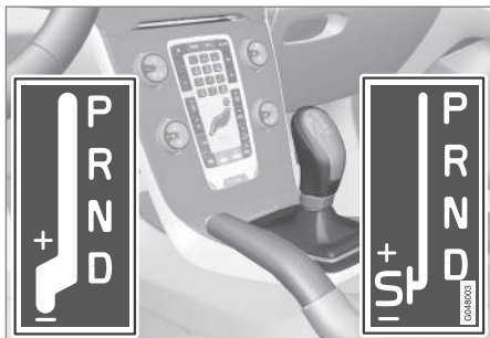
D: Automatic gear positions. +/-: Manual gear positions. S: Sport mode*. 12
