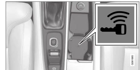
Location of the backup reader in the tunnel console.
