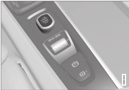
Start knob in the tunnel console.
