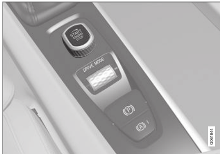
Start knob in the tunnel console.
