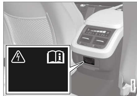
Electrical outlets in the tunnel console, rear seat.
