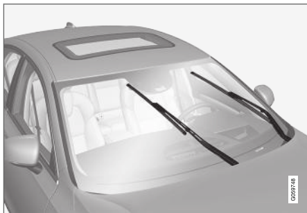
Viskerblader i servicestilling.
