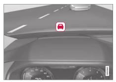
Collision warning symbol on the windshield<sup>57</sup>.
