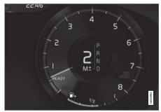
Manual shifting mode in the instrument panel<sup>2</sup>.
