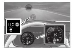
The previous illustration <sup>62</sup> shows that Pilot Assist is set to maintain a speed of 110 km/h (68 mph) and is following a target vehicle ahead that is traveling at the same speed.
