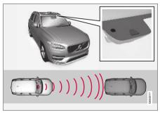
The camera/radar sensor measures the distance to the vehicle ahead<sup>37</sup>.
