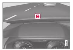
Collision warning symbol on the windshield<sup>39</sup>.
