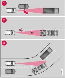
The radar sensor's field of vision.
