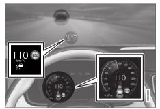
The previous illustration<sup>54</sup> shows that Adaptive Cruise Control is set to maintain a speed of 110 km/h (68 mph) and is following a target vehicle ahead, which is traveling at the same speed.
