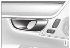
Alternative unlocking method using side door opening handle  $^{\rm 14}.$
