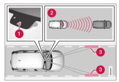
The camera/radar sensor monitors the distance to the vehicle ahead and detects lane markings<sup>55</sup>.
