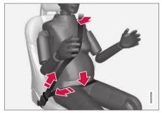
The seat belt should fit closely against the shoulder, with the diagonal section between the breasts and to the side of the stomach.
