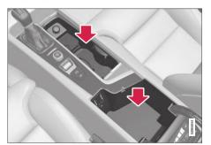
Storage compartments with cup holders, electrical outlets and USB ports in the tunnel console.
