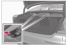
Fold down the hook from underneath the parcel shelf. Bags with handles of a suitable height can be hung from the hooks.
