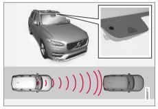
Location of the camera and radar sensor<sup>68</sup>.
