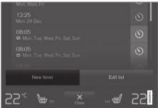
Button for adding a timer setting in the **Parking climate** tab in Climate view.
