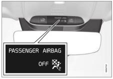
Occupant Weight Sensor (OWS) indicator light
