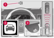
Collision warning audible signal and symbol<sup>38</sup>.
