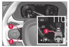
Controls for setting a time interval<sup>58</sup>.
