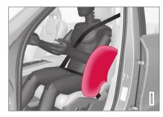
The side airbags are located in the front seats' outer backrest frames and help protect the driver and front seat passenger.
