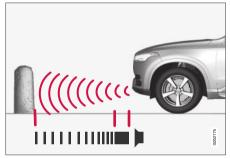
Continuous tone warning signal when the obstacle is less than approx. 30 cm (1 ft) from the vehicle <sup>113</sup>.
