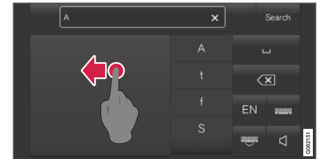
Delete all characters in the text field (2) by swiping across the handwriting field (1).
