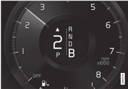
Gear shift indicator in the driver display 3 .
