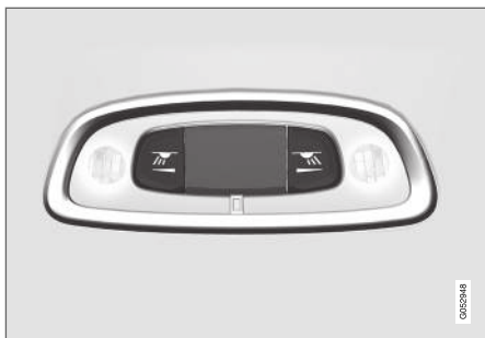
Reading lamps above the rear seat 6 .
