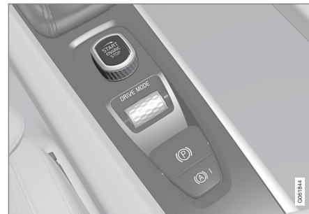
Start knob in the tunnel console.
