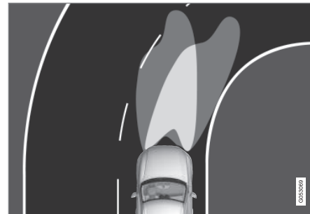
Headlight pattern with function deactivated (left) and activated (right).
