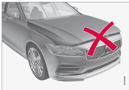
Hood not completely closed.
