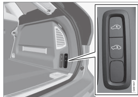
Controls for raising/lowering the car's rear section.
