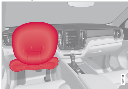
Steering wheel airbag and knee airbag 1 on the driver's side in the front seat.
