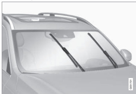
Viskerblader i servicestilling.
