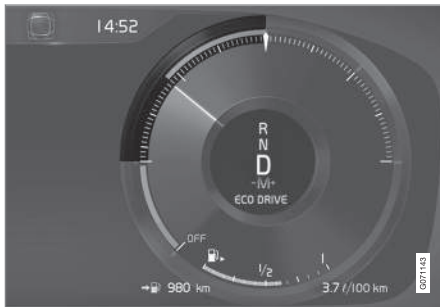
Eco gauge in 12" instrument panel*.
