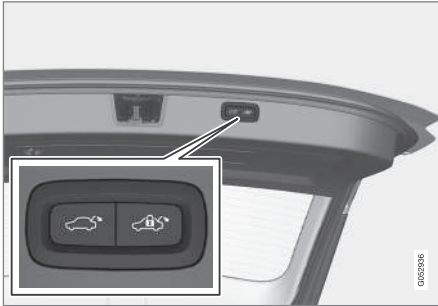
Location of button(s) on underside of tailgate.
