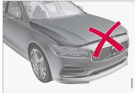
Hood not completely closed.
