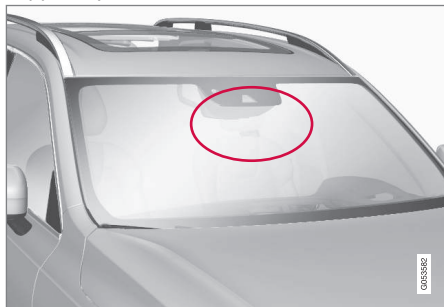
Location of radar sensor
