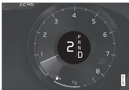
Instrument panel when shifting gears using steering wheel paddles, large gear selector.
