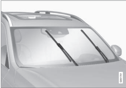
Windshield wipers in the service position.
